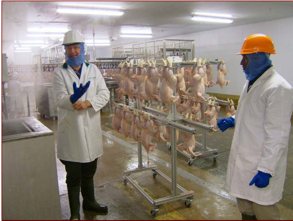
Figure 1. Rack in use in poultry processing plant (hot water rig at left).
