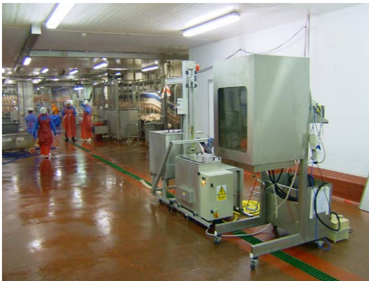
Figure 1. Atmospheric steam and hot water immersion pilot rigs at the poultry plant.
